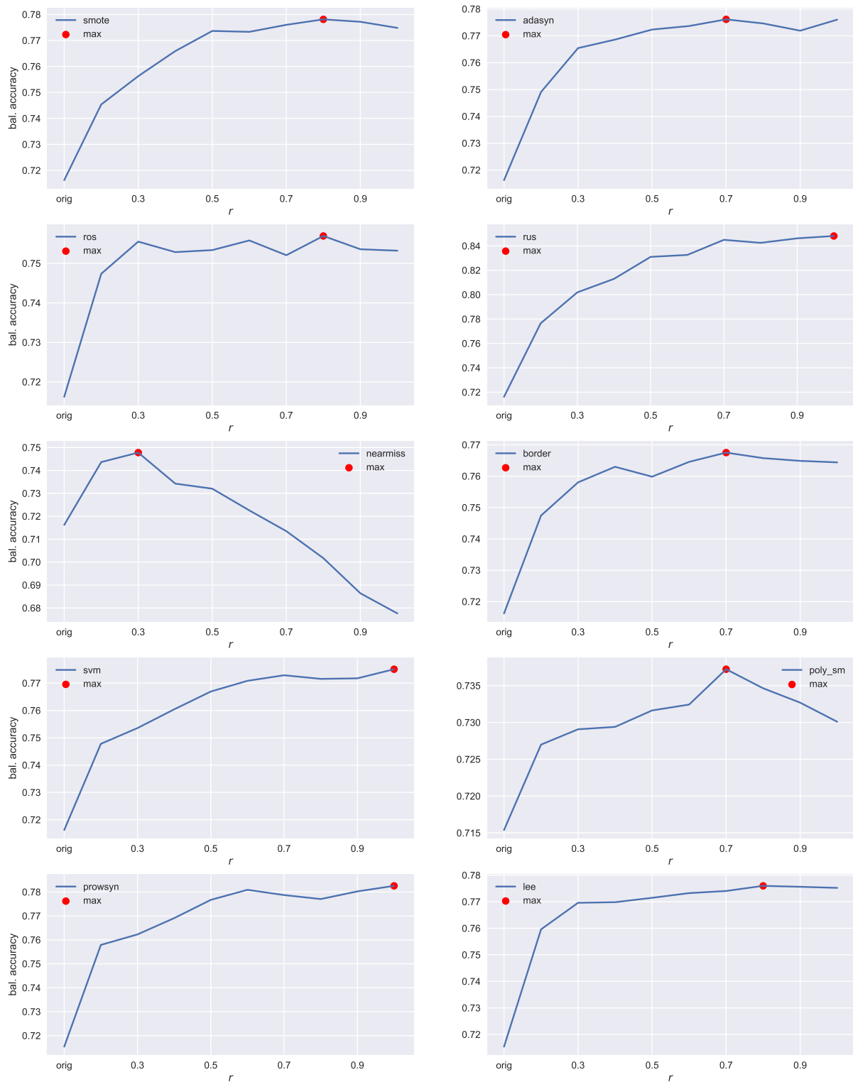
Figure 2: The mean accuracy of each sampling method, where the average is taken over all the datasets in Table 1. The accuracy is measured by the performance of the RF classifier trained on the sampled data.
